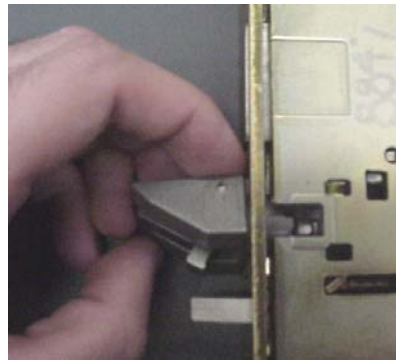
Step 4. Rotate Latchbolt 180 0 to desired handing position.
